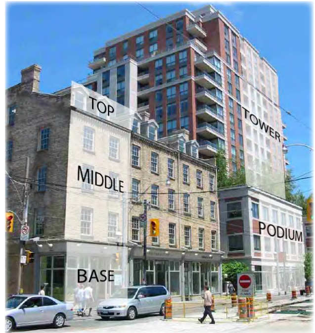
Each building should include a distinct base (storefront), middle (apartments or offices) and top (roof and penthouse) section.
