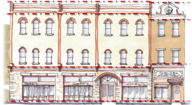
Vertical Articulation: Use cornices, window designs, materials, colours, sign bands, or other techniques to divide the building into base, middle and top sections.
