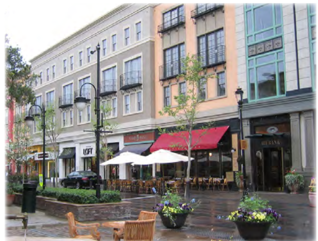
Example of one long building which has been visually broken down into smaller components through facade articulation, relief, and multiple storefronts.
